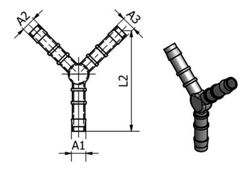
Ext. Hose Diameter A1 = 19 Ext. Hose Diameter A2 = 19 Ext. Hose Diameter A3 = 19 L2 = 72
